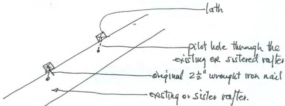
DETAIL OF "OBLIQUE HOLE" as a pilot hole for the stainless steel fastening screw.
