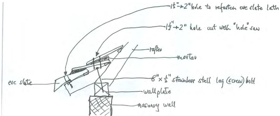
Fastening of False Rafter foot to Wall plate
