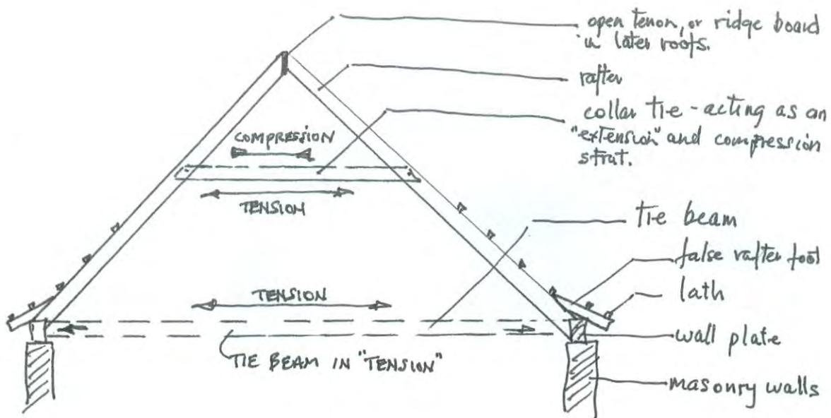
The collar tie acts both to stop the outward force on the masonry walls and, in compression, balancing the weight of the opposite sides of the roof against each other.
