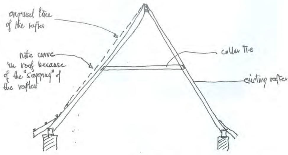
X-SECTION OF RAFTER SYSTEM OF BERMUDA ROOF
