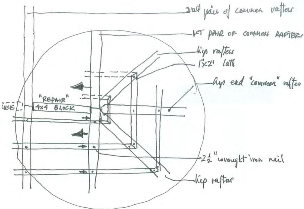
PLAN VIEW - JUNCTION OF HIP RAFTERS WITH COMMON RAFTERS
